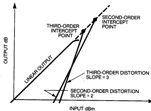
Figure 1. Receiver distortion vs. input power intercept point extrapolation (theoretical).
