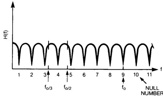
Figure 8. Frequency response of delay-line filter.
