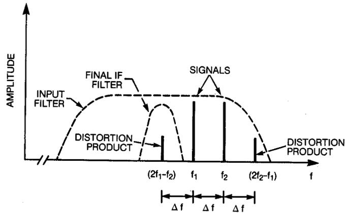
Figure 2. Third-order distortion products from two signals inside the receiver input filter.
