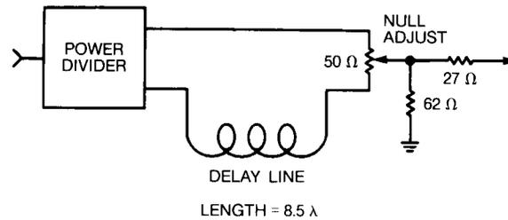
Figure 7. Delay-line notch filter.
