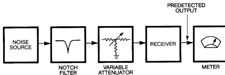
Figure 4. NPRFOM test configuration.
