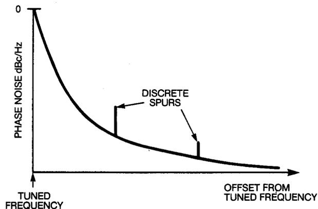
Figure 5. Receiver phase noise.
