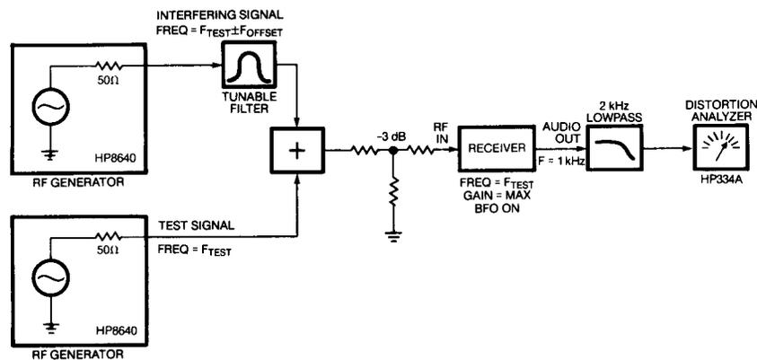
Figure 2. Desensitization dynamic-range test configuration.
