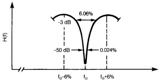
Figure 9. Detail of delay-line filter frequency response for ninth null.
