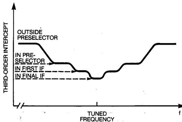
Figure 3. Third-order intercept as a function of test-tone frequency relative to receiver-tuned frequency.
