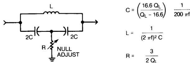
Figure 6. Notch filter with 6%, -3 dB bandwidth for 50-ohm source and load.
