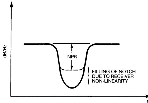
Figure 3. Noise power ratio (NPR).
