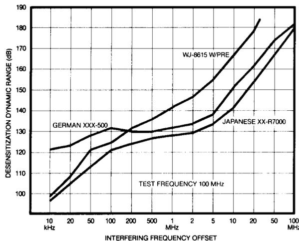
Figure 1. Desensitization dynamic range (DDR) as a function of frequency offset of the interfering signal.
