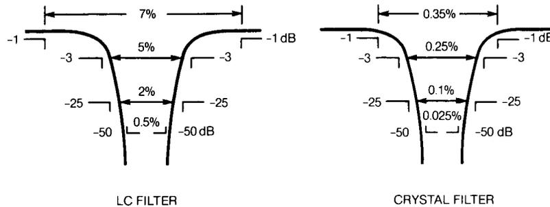
Figure 5. Recommended notch-filter bandwidths for NPRFOM measurements.
