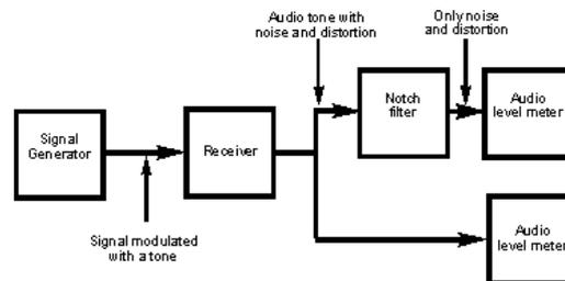
Figure 2 Making a SINAD measurement
