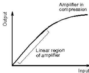
Fig. 1 A typical amplifier characteristic
