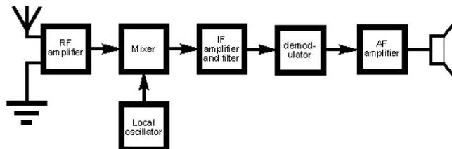
Figure 1 Block diagram of a basic superhet receiver
