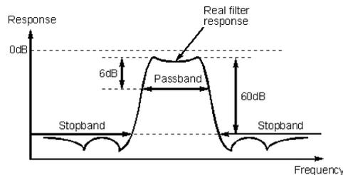
Figure 3 Typical response of a real filter
