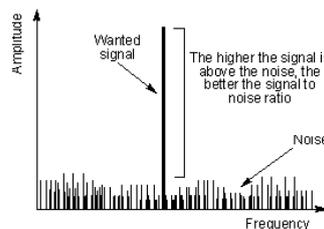
*Figure 1 Signal to noise ratio*
