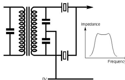
Figure 4 A basic half lattice crystal filter section
