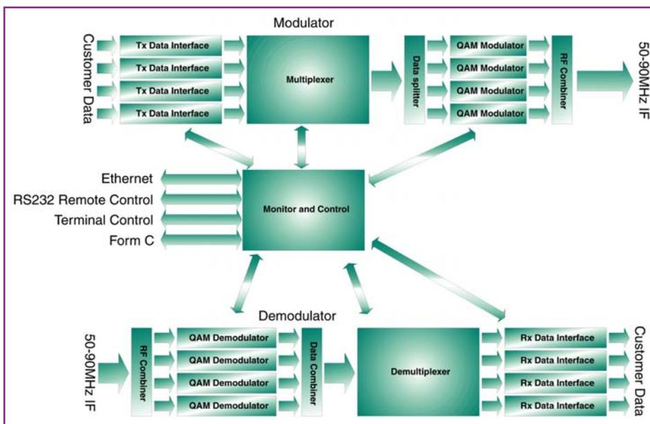
Figure 1. MM200 Functional Block Diagram
