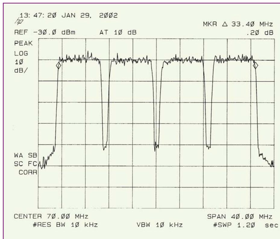
Figure 5. MM200 Typical Output Spectrum
