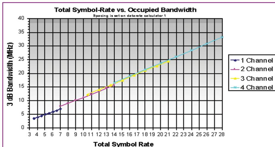
Figure 7. MM200 Total Symbol Rate vs. Occupied Bandwidth
