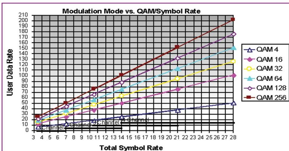
Figure 6. MM200 Modulation Mode vs. QAM/Symbol Rate
